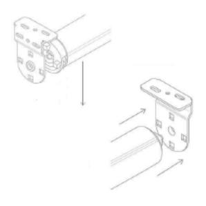
Hold the fully wound blind, insert the idle pin end into the bracket as shown.
