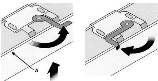
Push the swing arm anti-clockwise as far as it will go to 'open' the bracket.
