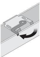
Push swing arm clockwise until it locks in to place, firmly holding the blind headrail.
