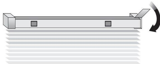
Push down and snap the hinge doors shut to lock the headrail into position.
