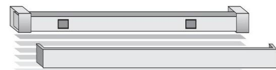
If you have selected an 'Exact' measurement, your blind will be supplied with pelmet returns. These can be attached on to the sides of the brackets using velcro patches in the same way.
