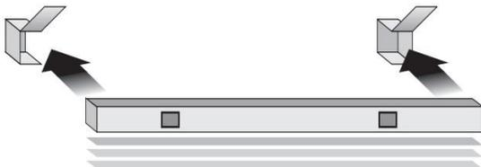
Once the brackets are fitted, remove the plastic end caps from the blind headrail.
