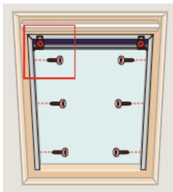
NB. Once the side channels are screwed in place, you should see that there are no gaps around the headbox and channels.
