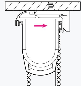
Then simply hook the front of the head rail over the front of the bracket. Once hooked in at the front push the back of the bracket up to level out the head rail then push back until you hear it click into place.
