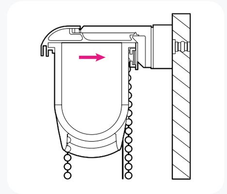
Then simply hook the front of the head rail over the front of the bracket. Once hooked in at the front push the back of the bracket up to level out the head rail then push back until you hear it click into place.
